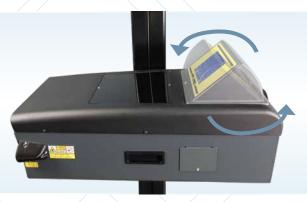
Rotating display for easier projector adjustment Green laser for vehicle alignment
